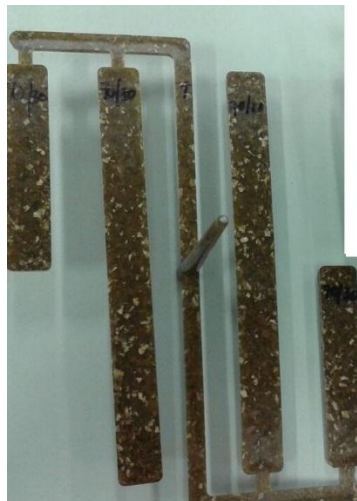
Figure 3 - 7 : Specimen for impact and flexural test
