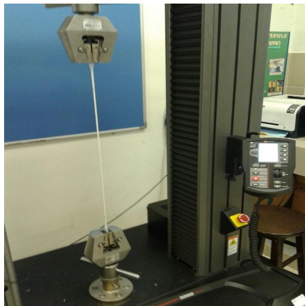
Figure 3 - 9 : Tensile testing for neat Polypropylene.
