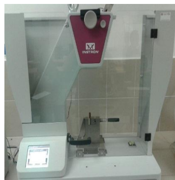
Figure 3-14: Izod Impact testing machine.
