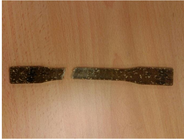
Figure 3 - 10 : Specimen break after tensile test.
